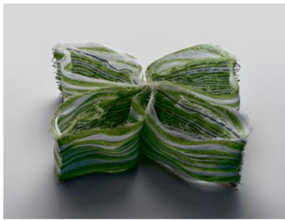
Entangled: Functional textiles that change shape and react to light and temperature. Photo: Bryan Saragosa
